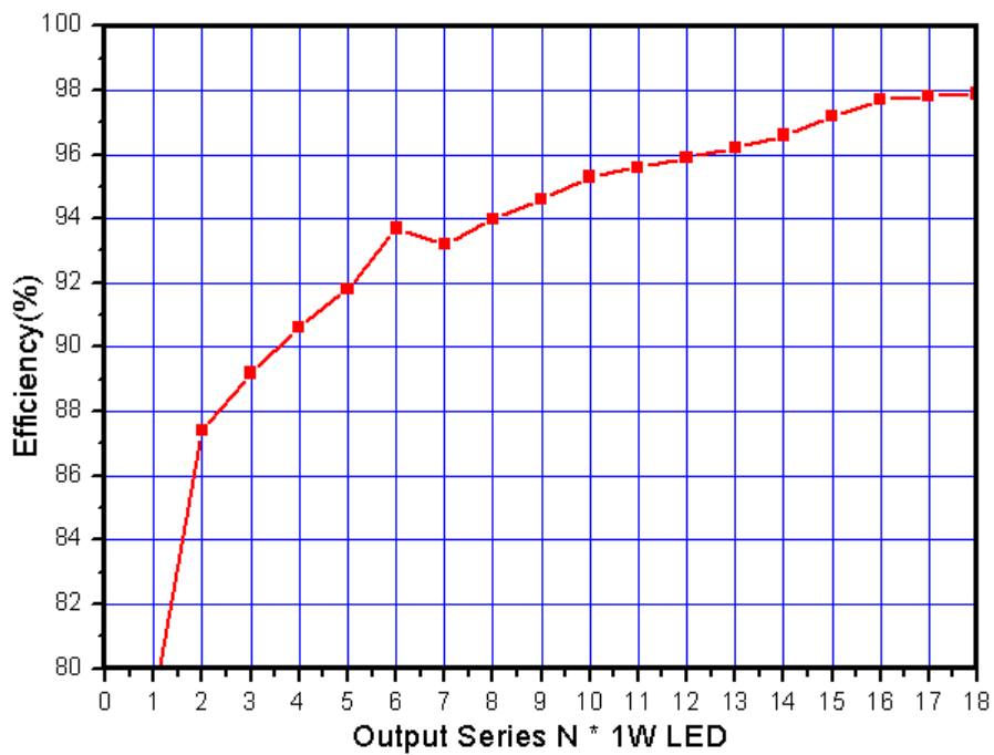
Figure5. Efficiency VS Output N*1W LED
